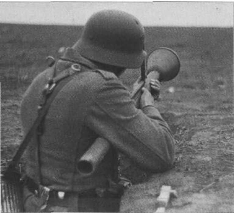
Above: The Panzerfaust 30 was the simplest of all German rocket-propelled grenade launchers. Its designation referred to its optimum range - 30m (32.8 yards).
